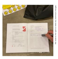
Use the permanent marker (included in the inspection kit) to mark the month and year for the next inspection. Write your name and the date of the current inspection underneath the sticker.
