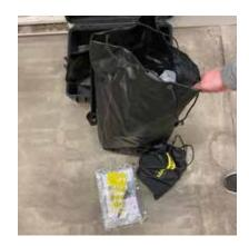
3. Make sure that the Sealpac is not punctured or othervise affected. The Sealpac should look like in the left picture. If the Sealpac looks like the pack in the right picture it has been punctured or othervise affected, and lost its function. If this is the case it needs to be sent to SafetyRespect for full inspection and resealing.
